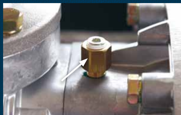
Vent ports to alleviate vapour lock and help with priming
